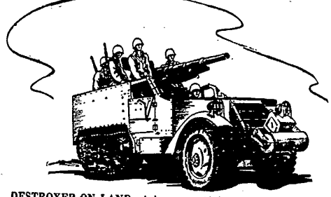
DESTROYER ON LAND—A heavy, rapid-fire cannon mounted on a half-track armored car, that's the self-propelled artillery, the answer to the Armed Forces' need to thrust heavy artillery firepower directly into the core of its lightning attacks.
